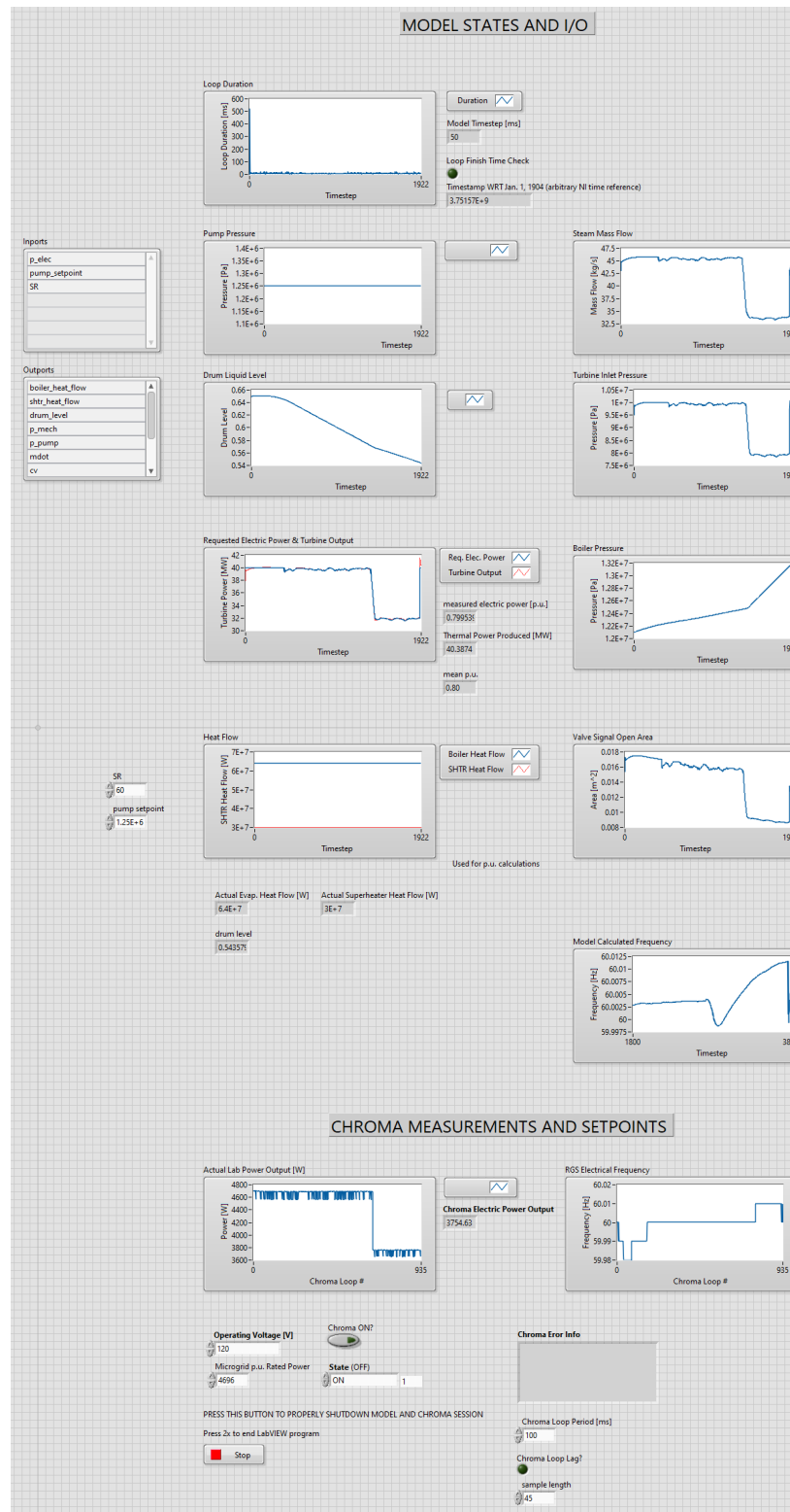
Figure 3.33: PC 1 front panel in LabVIEW . All inputs and outputs can also be found in the Simscape model Fig. 3.2
